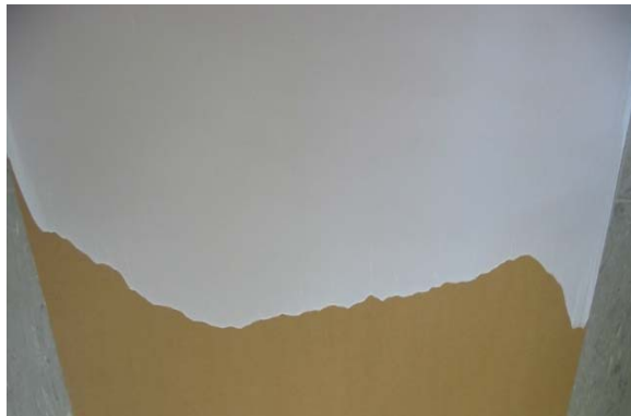
Fig. 5: Coverage with curtain coater on brown substrate
