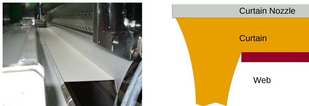
Fig. 11: “Overboard” mode for curtain coater: Curtain wider than web
