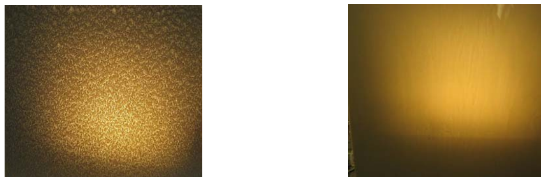
Fig. 11: Coating color on a glass plate - Visualization of air before and after deaeration (no magnification)
