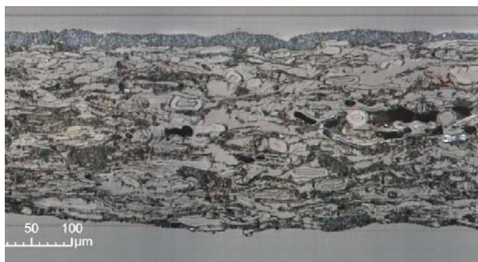
Fig. 12: Scanning electron microscopy of samples coated with air knife.
