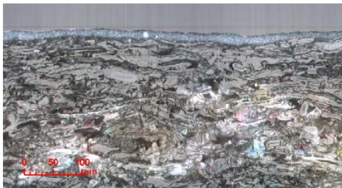
Fig. 13: Scanning electron microscopy of samples coated with curtain coater.
